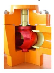
The ball has rotated the full 90 degrees without touching the seat.
