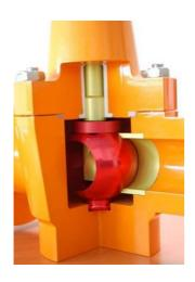
As the stem continues to lower, a flat angled surface (helix top part) forces the ball to wedge mechanically against the metal seat to ensure proper seat tightness.
