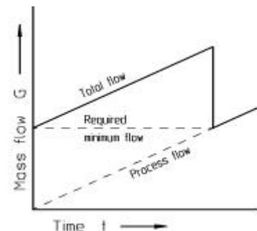
**Fig. 6:** On/Off Operation
