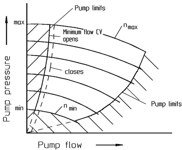
Fig. 12: Characteristic curve for an speed controlled pump
