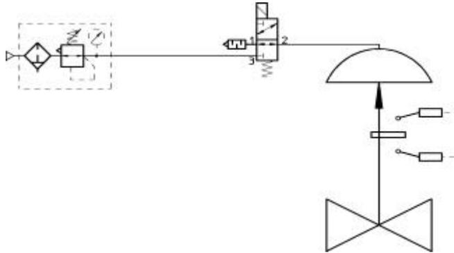
Fig. 10: Diagram on/off operation
