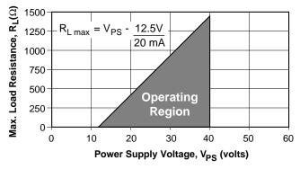
**Figure 3: Power Supply Requirements**
