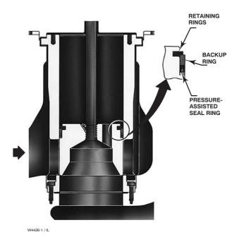
Figure 14. Fisher® EHT Trim (NPS 8 through 14 Globe Valves)
