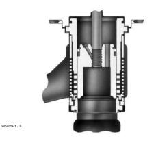
Figure 10. Fisher® EHAT Trim (NPS 3 through 8 Angle Valves)
