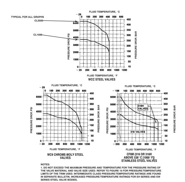
Figure 26. Pressure/Temperature Limits for CL1500 and 2500 Valves (NPS 8 through 14 Valves)
