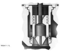
DIVERTER CONE VALVE PLUG USED FOR  $\Delta P\!\!>\!3000$  PSI (207 BAR) OR FOR WHISPER TRIM III LEVEL A, B, OR C CAGES
