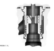
Figure 9. Fisher® EHAD Trim with Whisper Trim® III Level D Cage
