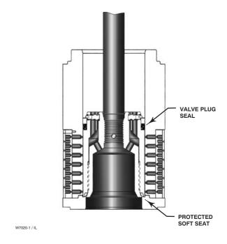
Figure 23. Typical Balanced TSO (Tight Shutoff) Trim
