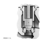
Figure 6. Fisher® EHS Trim with Micro-Form Valve Plug
