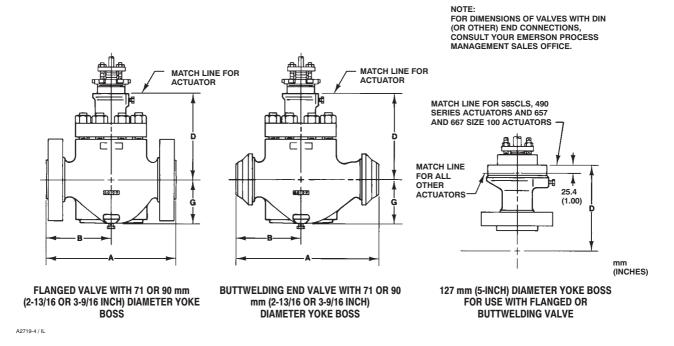
Figure 28. NPS 1-1/2 x 1 through 6 Globe Valve Dimensions with Standard Bonnet (also see tables 24, 25, and 26)
