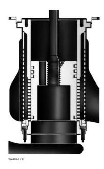
Figure 15. Fisher® EHD Trim with Whisper Trim® III Level D Cage (NPS 8 through 14 Globe Valves)
