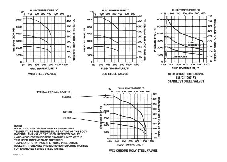
Figure 24. Pressure/Temperature Limits for CL2500 Valves (NPS 1-1/2 x 1 through 6 Globe) and CL900, 1500, and 2500 Valves (NPS 3 through 8 Angle)
