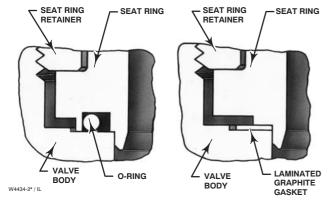
O-RING GASKET CONSTRUCTION, STANDARD CONSTRUCTION FOR EHT, CAVITROL TRIMS, AND SOUR SERVICE
