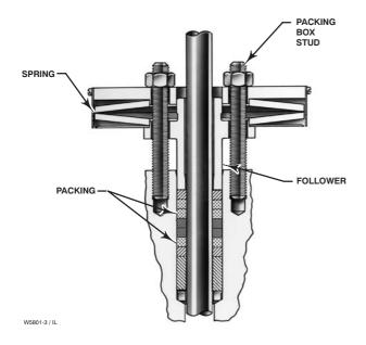
Figure 2. Typical HIGH-SEAL Packing System
