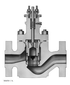
Figure 5. Fisher® EHD Valve Body Assembly
