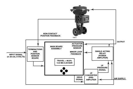
Figure 3. DVC2000 Series Digital Valve Controller Block Diagram
