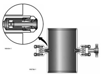
Figure 4. Design TBX-T Desuperheater
