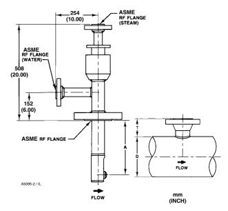
Figure 10. Design DSA Dimensions (also see table 3)
