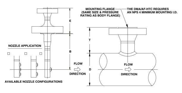
Figure 12. Design DMA/AF-HTC Dimensions (also see tables 5 and 6)
