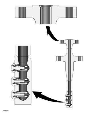
Figure 5. Design DMA/AF-HTC Desuperheater
