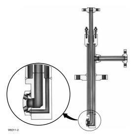
Figure 3. Design DSA Desuperheater
