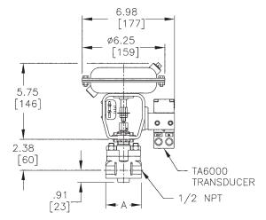
Figure 9. Type 16 Actuator Front
