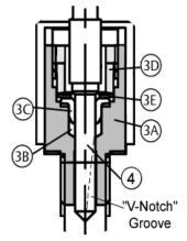
Figure 6. Soft Seat Cage Assembly
