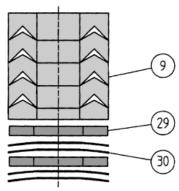
Figure 7. V-Ring Packing Kit
