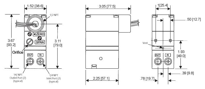
Figure 11. TA6000 Electropneumatic Transducer Dimensions, inches [millimeters]
