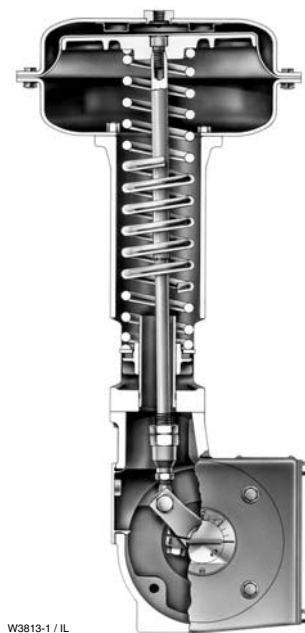
Figure 3. Sectional Views Typical of Size 40, 60, and 70 Actuators
