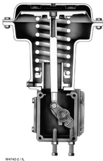
Figure 4. Sectional Views of the Size 33 Actuator
