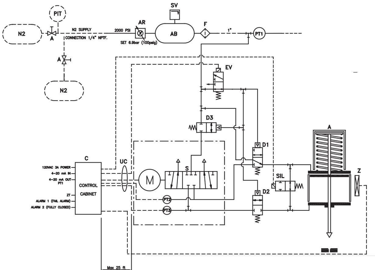
**Fully Customizable, Zero Bleed, Remote Location Schematic**
