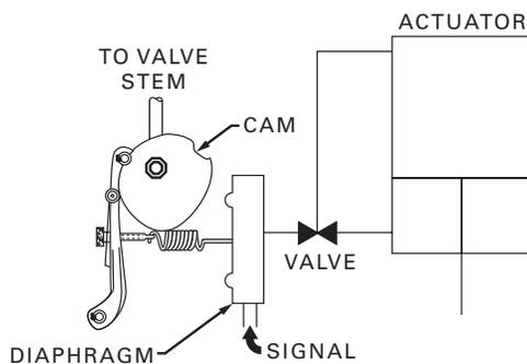
Figure 2: Operational Schematic
