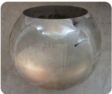
兖矿国泰锁渣阀维修
